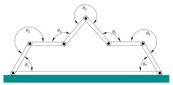
Figure 7.23: A chain of links in the plane. There are seven links and seven joints, which are constrained to form a loop. The dimension of C is seven, but the dimension of  $C_{clo}$  is four.
