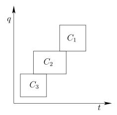
Figure 7.2: Transitivity is broken if the cells are not formed in cylinders over T. A time-monotonic path exists from  $C_1$  to  $C_2$ , and from  $C_2$  to  $C_3$ , but this does not imply that one exists from  $C_1$  to  $C_3$ .
