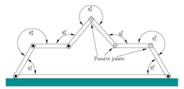
Figure 7.24: Three of the joint variables can be determined automatically by inverse kinematics. Therefore, four of the joints be designated as *active*, and the remaining three will be passive.
