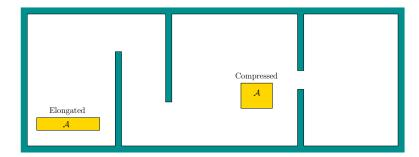
Figure 7.13: An example in which the robot must reconfigure itself to solve the problem. There are two modes: *elongated* and *compressed*.
