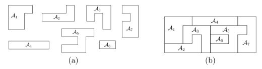
Figure 7.7: (a) A collection of pieces used to define an assembly planning problem; (b) assembly planning involves determining a sequence of motions that assembles the parts. The object shown here is assembled from the parts.
