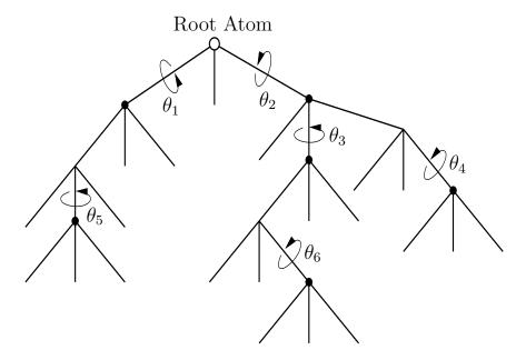
Figure 7.33: The modeling of a flexible molecule is similar to that of a robot. One atom is designated as the root, and the remaining bodies are arranged in a tree. If there are cyclic chains in the molecules, then constraints as described in Section 4.4 must be enforced. Typically, only some bonds are capable of rotation, whereas others must remain rigid.
