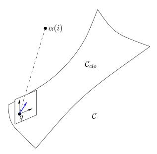
Figure 7.22: For each sample  $\alpha(i)$  the nearest point,  $q_n \in \mathcal{C}$ , is found, and then the local planner generates a motion that lies in the local tangent plane. The motion is the project of the vector from  $q_n$  to  $\alpha(i)$  onto the tangent plane.
