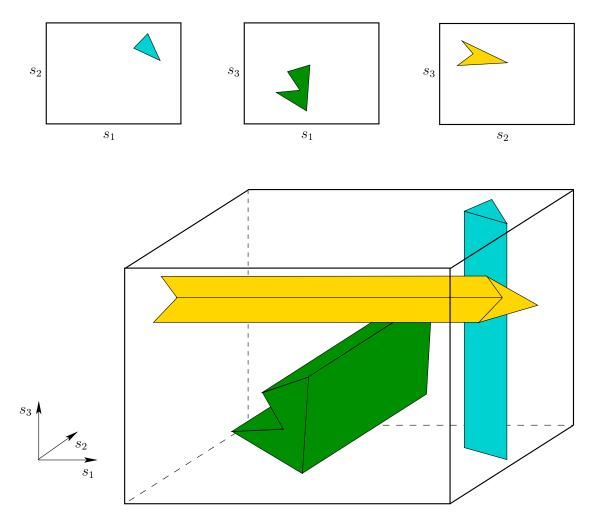
Figure 7.9: The obstacles that arise from coordinating m robots are always cylindrical. The set of all  $\frac{1}{2}m(m-1)$  axis-aligned 2D projections completely characterizes  $X_{obs}$ .
