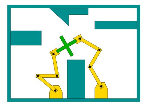
Figure 7.19: Two or more manipulators manipulating the same object causes closed kinematic chains. Each black disc corresponds to a revolute joint.
