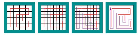
Figure 7.38: A circular path is made by doubling the resolution and following the perimeter of the spanning tree.
